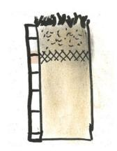
Before tilling intervention, carry out a spade test to assess the condition of the subsoil (see explanations and sample images). Only work as deeply and intensively as necessary for the current crop. Vary the depth of tillage depending on the crop. Use an onland plough, avoid smear layers (e.g. with a rotary tiller) or compaction of the soil aggregates during tillage in too moist soil (e.g. with a roundabout harrow).
